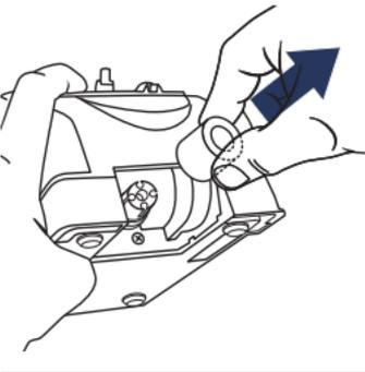
4. Remove worn wheel by twisting slightly and lifting wheel off shaft. Install new wheel and reinstall wheel retainer and screw. Don't over-tighten mounting screw (tighten to about 48 in/lbs). Remove the wrench and replace the Wheel Access Cover before turning on the machine.
