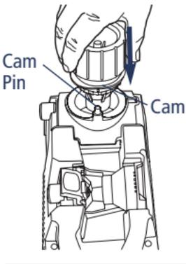
Line up the Sharpening Guide (white lines) on the Chuck with the Cam Pin on the machine. Plunge the Chuck into the Sharpening Port until it touches the Sharpening Wheel. Remove the Chuck, rotate one half-turn clockwise and repeat. Inspect the bit and continue until the cutting surfaces are sharp. If the bit stops grinding before the edges are sharp, reset the depth and sharpen some more.
