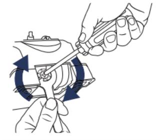
3. With #3 Phillips head screwdriver, remove one left-handed screw (clockwise to loosen) and remove the wheel retainer.
