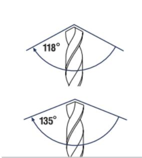
Most bits are 118° or 135°. Hold your bit point up to the key to the left to see which type your bit looks like. Most wood and soft metal applications require 118°. Harder materials such as stainless steel and tool steel require 135°. If you are drilling contoured materials (such as a car fender), plan on splitting the point to prevent walking of the bit.
