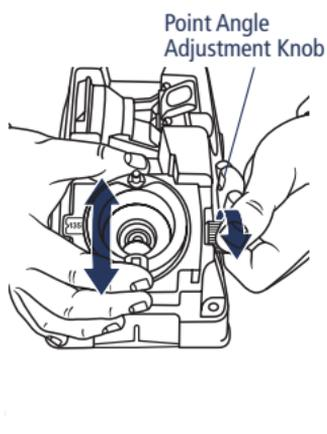
The Model DD750X has additional advanced features that enable you to fine-tune your bit geometry. Loosen the Point Angle Adjustment Knob to the right of the Sharpening Port and slide the metal Point Angle Adjustment Plate to standard 118° or 135° (or anywhere in-between, allowing you to create the custom angle of your choice.) Choose the point angle based on the application (material) you're drilling. Then re-tighten the Knob.
