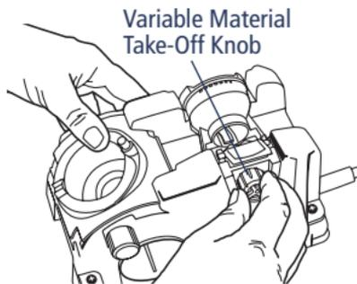
The **Model DD750X** enables you to remove more or less material from the tip of your bit when you sharpen. If your bit is only slightly dull and you simply wish to “touch up” its point, turn the Material Take-Off (MTO) Knob **clockwise** to reduce the amount of material that is
