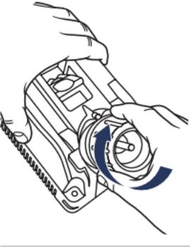
Different size drill bits may require a different number of rotations. Continue to sharpen until you no longer hear grinding noise. This will result in a Chisel Edge that is clean and straight and ensure the entire surface from the Cutting Edge to the Heel is finely ground.
