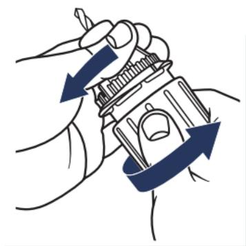
Press the Alignment Button and remove the Chuck from the Alignment Port. Tighten the Chuck once more to ensure the bit won't move when you sharpen it.
