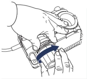
Hold onto the Chuck and tighten the Chuck Knob until it is snug. (Avoid over-tightening the Chuck in the Alignment Port as this could damage the alignment teeth in the port.)
