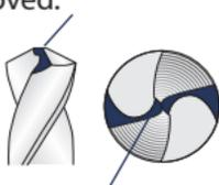
Split lines are joined in the center and Chisel edge has been removed.
