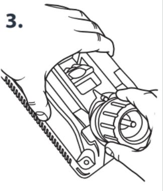
Each notch in the Alignment Port is approximately a 10° change in Chisel Angle.
