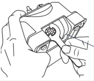
2. Use wrench supplied with your Drill Doctor to hold sharpening wheel in place.
