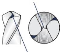
Not enough material has been removed from the Heel of the drill bit.
