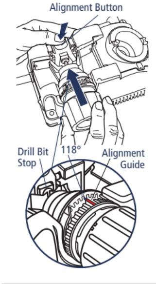
Press the Alignment Button down that opens the bit clamp arms. Insert either of the Alignment Guides (raised fins) on the Chuck into the 118° notch on the Alignment Port. With the clamp arms held open, slide the drill bit forward until it touches the Drill Stop. (Make sure the Chuck is seated all the way into the Alignment Port). Now release the Alignment Button, releasing the clamp arms.
