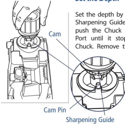
Set the depth by lining up one of the Sharpening Guides with the Cam Pin. push the Chuck into the Sharpening Port until it stops and tighten the Chuck. Remove the Chuck to ensure the insert is aligned with the Masonry Sharpening Marks and tighten again.
