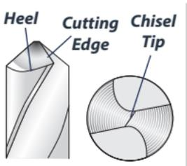
The entire surface from the Cutting Edge to the Heel will have a finely ground surface without indentations. The Heel will always be lower than the Cutting Edge (positive relief).
