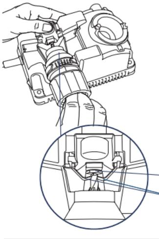
Check to ensure your bit is held in place correctly. The Clamp Arms should be holding the drill bit at its narrowest spot (in the flutes). If they aren't, turn the bit slightly until they fall into the flutes. This is an important step to proper alignment.
