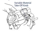
The **Model DD750X** enables you to remove more or less material from the tip of your bit when you sharpen. If your bit is only slightly dull and you simply wish to "touch up" its point, turn the Material Take-Off (MTO) Knob **clockwise** to reduce the amount of material that is
