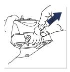
4. Remove worn wheel by twisting slightly and lifting wheel off shaft. Install new wheel and reinstall wheel retainer and screw. Don't over-tighten mounting screw (tighten to about 48 in/lbs). Remove the wrench and replace the Wheel Access Cover before turning on the machine.
