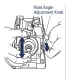
The Model DD750X has additional advanced features that enable you to fine-tune your bit geometry. Loosen the Point Angle Adjustment Knob to the right of the Sharpening Port and slide the metal Point Angle Adjustment Plate to standard 118° or 135° (or anywhere in-between, allowing you to create the custom angle of your choice.) Choose the point angle based on the application (material) you're drilling. Then re-tighten the Knob.
